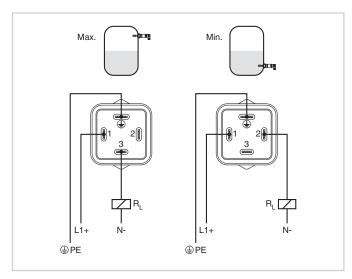
VEGASWING 53 with valve block according to ISO 4400
