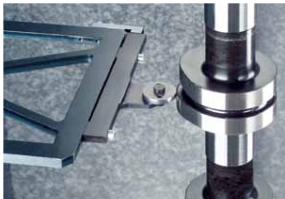
Round measuring follower made of different materials for cam shaft diameters
