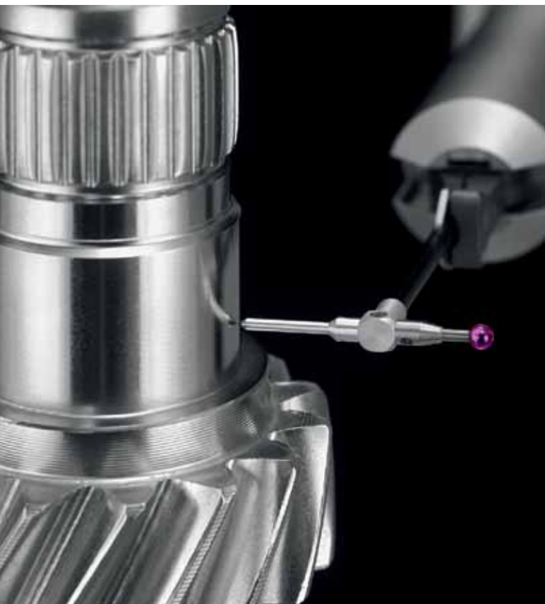
Twist measurement with a roughness stylus tip
