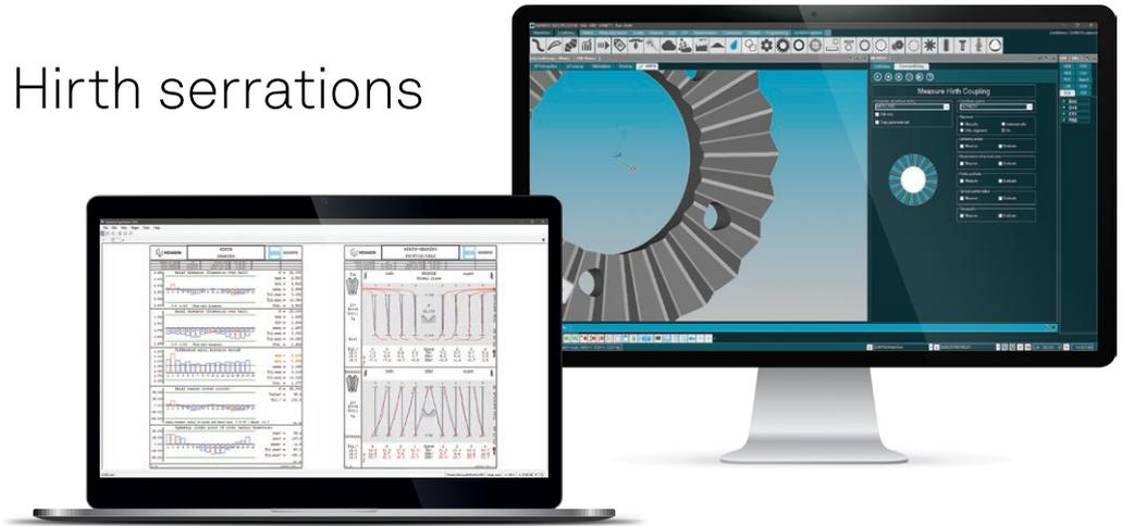
Hirth serrations are a specific type of plank serration, characterised by radially arranged teeth with a tapered symmetrical profile and flat tooth tips. This design ensures high torque stability, repeatability, and accuracy in terms of axial and radial runout. The tooth tip can also be inclined to the coupling axis for specific applications.
