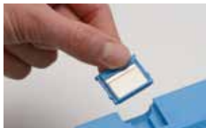
Integrated roughness standard
