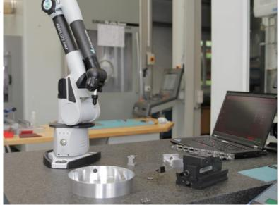
\*because this arm has counter weight instead of counter balance, it doesn't create torque, as the back and front sides are balanced. That means the arm will not move when you start your measurement.
