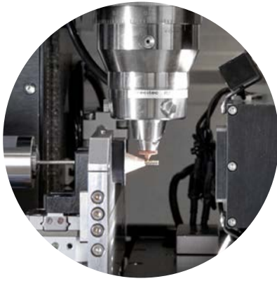
Special-designed spindle for very small delicate tube handling
